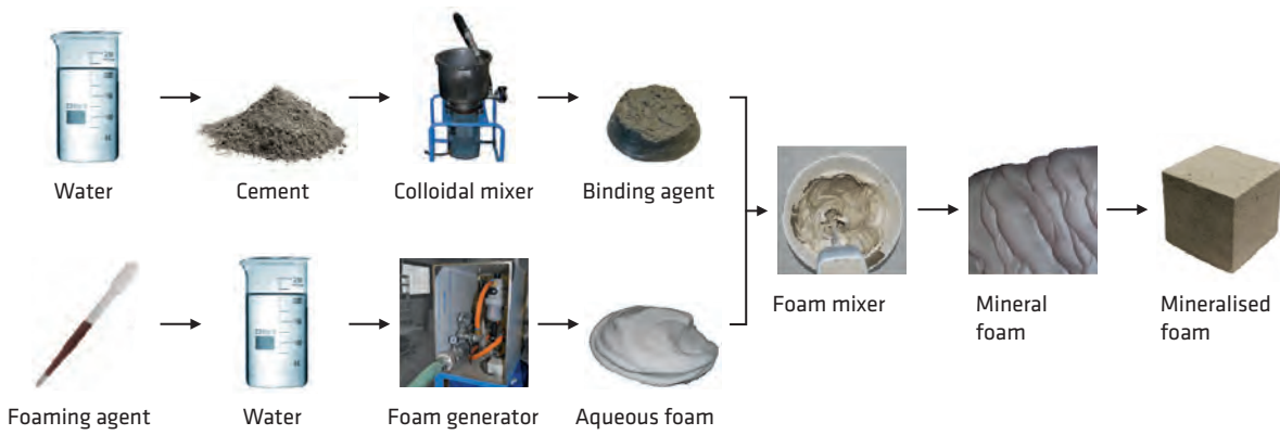
04 Manufacturing process of mineralised foam in a semi-continuous process
